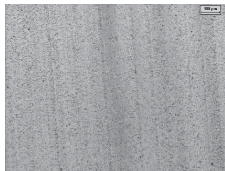
Figure 16. PHB/safflower 95/5. A well dispersed system is observed. POM 5X.
