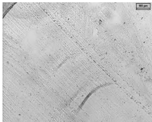
Figure 11. PHB/CAEI 80/20, 9 min mixing. Well dispersed blend with knife marks from the cutting process. POM 5X.
